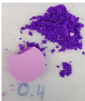
Fig. S19. Image of 0.4-ZIF-new, revealing a rich purple phase and a lighter phase being separated during the drying process.
