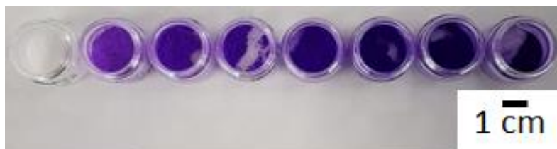
Fig. S1. Image of Co/Zn-ZIF-62 samples (from the left 0.0, 0.1, 0.2, 0.4, 0.6, 0.8, 0.9, 1.0) revealing the change in the intensity of the purple colour with increasing cobalt content.
