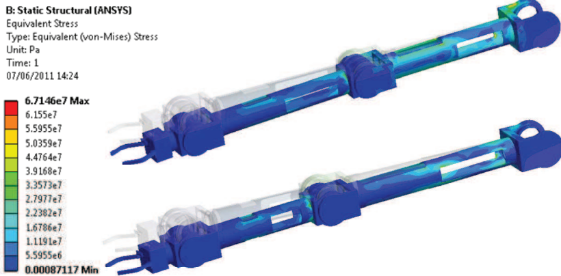
Figure 5.13: von-Mises element stress in the original (top) and optimized (bottom) robotic arms.
