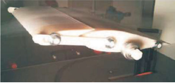
Figure 2. Double element airfoil in wind tunnel. (This figure is available in colour online.)
