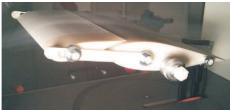
Figure 3.6 DU06-W200 double-element airfoil in the wind tunnel
