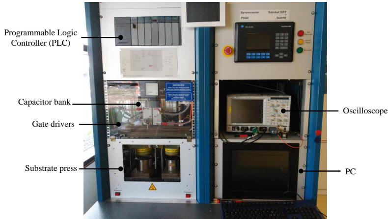
Figure 2.5: Picture of the dynamic substrate test bench at ABB for performing short-circuit tests.
