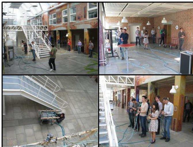
Fig. D.2: Several distributions of the users, spread or grouped, in LoS or NLoS, or without users. Top-left, S-LoS \parallel . Top-right, S-NLoS. Bottom-left, F-InFront. Bottom-right, G-LoS
