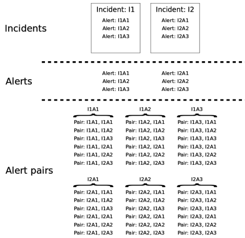
Fig. 4.3: The data used for evaluation consists of multiple traffic traces, two in this example. Each traffic trace corresponds to an infection and can be used to generate a set of IDS alerts. By pooling all alerts together and pairing all alerts with all alerts, a data set of pairs is obtained (Similar to a full outer join or Cartesian product).
