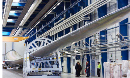
(d) Finished wind turbine blade (except for surface treatment).
