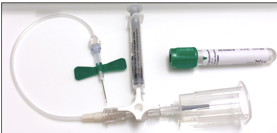
Figure 7. Blood gas sampling kit in the methodological pre-study in Study A. The three-way stopcock was attached to the standard sampling kit for uniform and rapid sampling.
