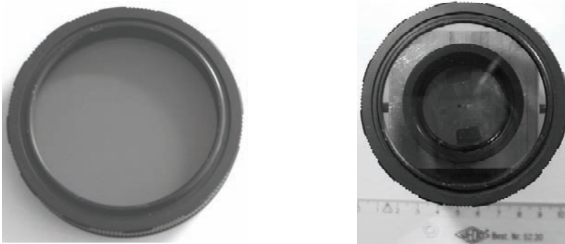
Figure H-6 The interference filter is placed in front of the optical set-up.
