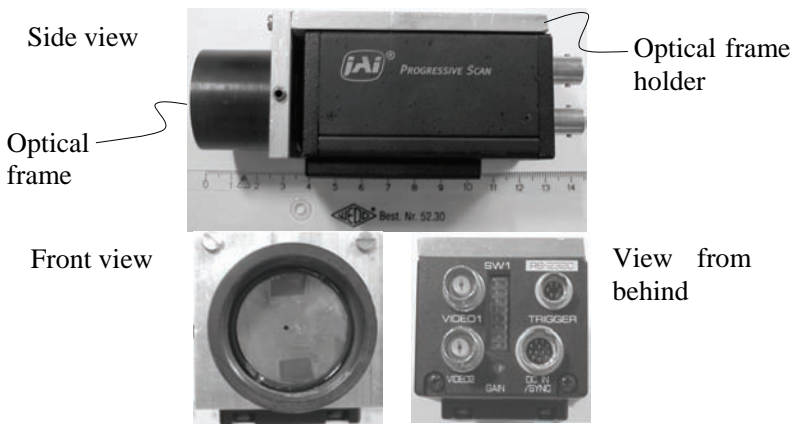
Figure H-3 The CV-M10 RS Progressive Scan Monochrome camera with the optical frame mounted.
