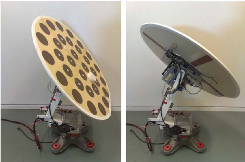
Figure 1.1: F77, SpaceCom's satellite tracking antenna.
