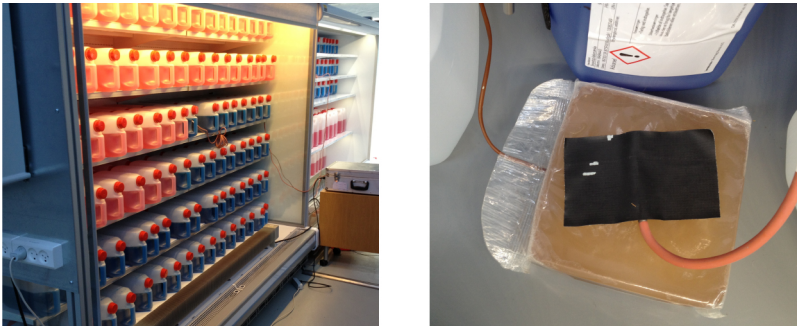
Figure 2.5: MT open shelving units with ethylene- and propylene-glycol containers (left) and tylose block with temperature sensors (right).
