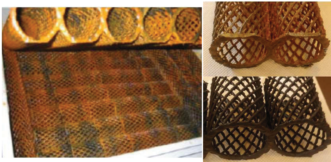
Figure 17 Pictures of iron hydroxides coated (BB-FeO) and clean (BB) polymer grid pipe
