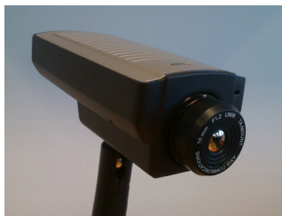
Fig. 2.7: Example of an uncooled thermal camera, AXIS Q1921.
