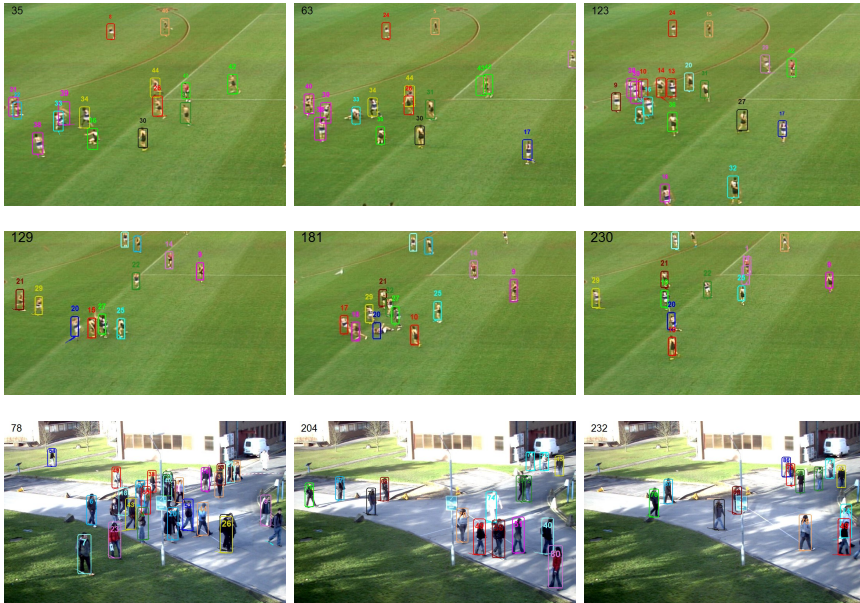
Fig. 10.5: Exemplar frames from two AFL clips and the PETS S2L2 sequence. Note that using model-free trackers allows one to maintain the identity of a player even during severe deformations and pose changes ( cf. the blue target (ID 20) in the second row).
