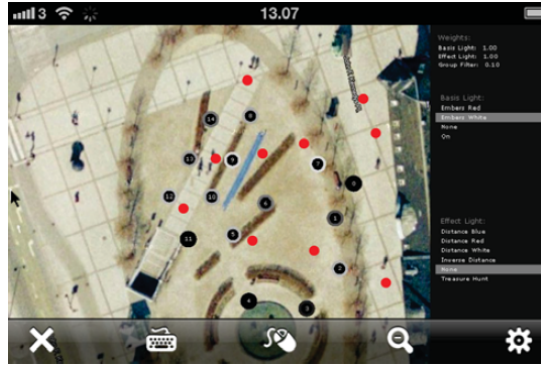
Fig. 12.5: Snapshot of the iPhone application by which it was possible in real-time to see the result of the computer vision tracking and the resulting control of lamps. It was also possible to manually control the lamps by the application.
