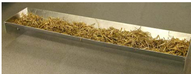
Fig. 2. Right angle gutter applied for long pile mass reduction of cut and particulate wheat straw. The gutter had two working positions: an upright (the one seen), applied when pouring the sample and a tilted (90°), applied for sample extraction.
