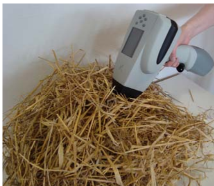
Fig. 1. Handheld NIR on straw - the ultimate solution for compositional characterization of straw.
