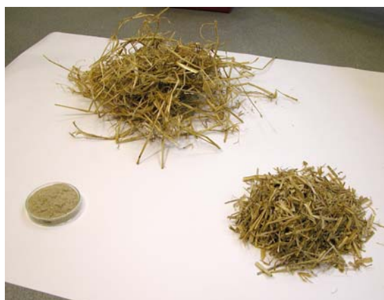
Figure 6.6: Wheat straw size after size reduction in first and second mass reduction (and comminution) steps.
