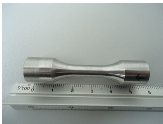
Figure 4-2 The fatigue test sample
