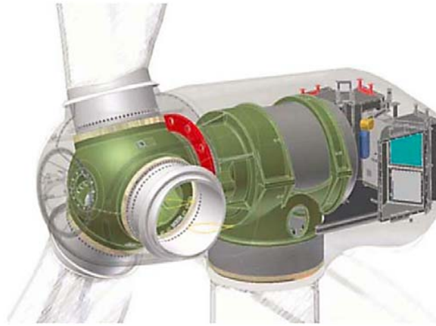
Figure 34: 10[MW]HTS Direct Drive Wind Turbine [102]
