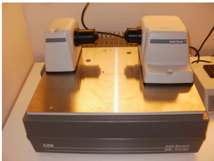
Figure 8.0: photograph of the NIRS equipment used for the analysis of the backwash precipitates.
