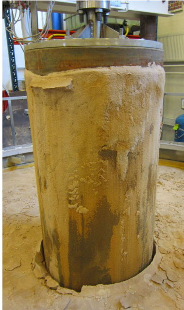
Figure C.5: Uninstallation of the pile after a test with applied suction. Sand is not resaturated before uninstallation, and some sand is stuck to the upper one third of the pile.
