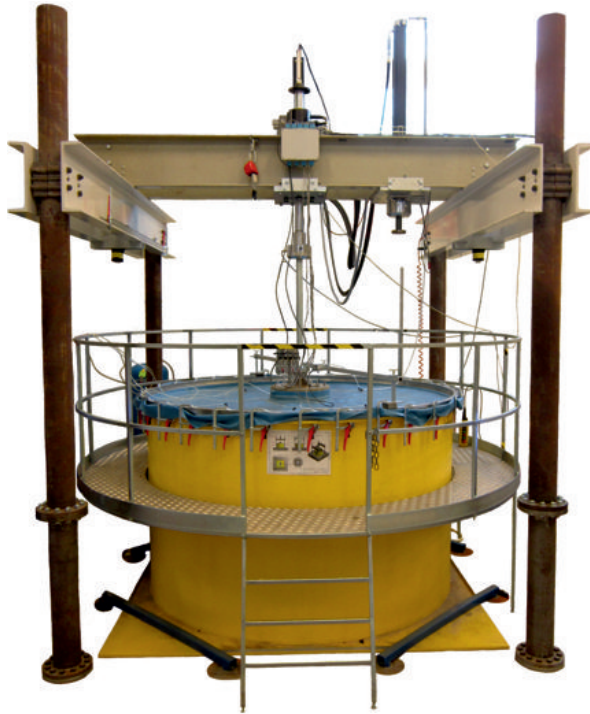
Figure C.2: Setup for a test with applied suction.
