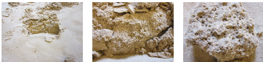
Figure 4.5: Sand structure after tests with applied suction.
