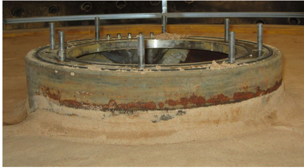
Figure C.4: After tests with applied suction, sand in the interface is stuck to the pile.
