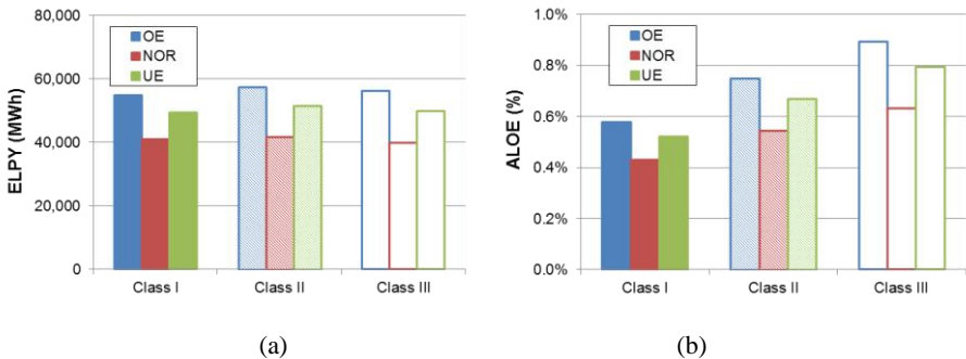
Fig. 5.7. Cost of energy with different wind classes. (a) Energy Loss Per Year (ELPY); (b) Annual Loss Of Energy (ALOE).
