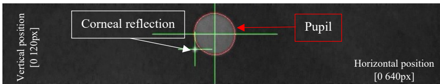
Figure 3-5. An eye image with the detected pupil (red circle) and corneal reflection (CR).
