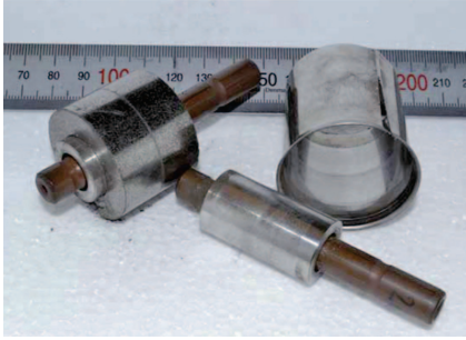
Figure 1.2. Dismantled rotor container [18].
