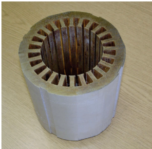
Figure 1.14. Stator made of amorphous laminations [48].
