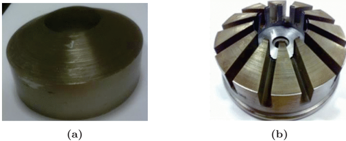
Figure 1.18. AFM rotor structure; (a) uncut, (b) cut [52].
