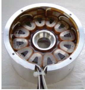
Figure 1.19. AFM with wounded amorphous stator cores [53].
