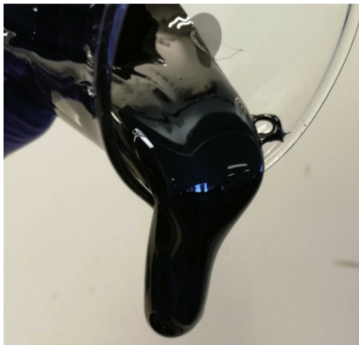
Fig. 1. Dehydrated and demineralized bio-crude (23 °C) used as feed in the sCO 2 extraction runs.
