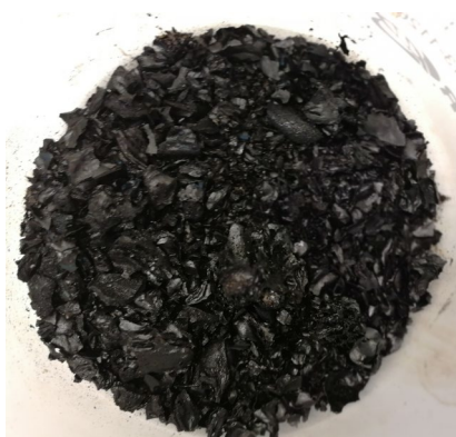
Figure 5.17: Example of sCO 2 residue. Extraction of BCR-DM at 120 °C and 248 bar.
