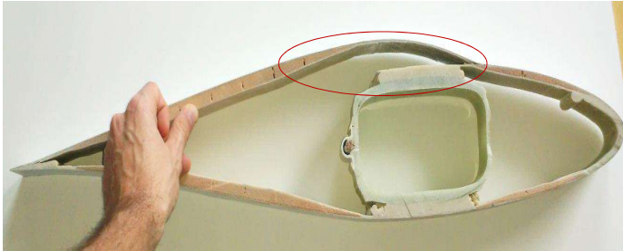
Fig. 1.10: Buckling can cause high peeling stresses and thereby skin debonding. Adapted with permission from Find Møhlolt Jensen, Bladena.
