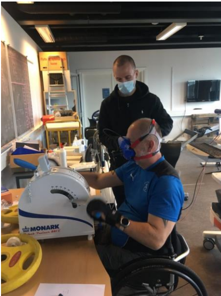
Figure 4. Participant performing a GTX for determination of \dot{V}O_{2peak} . The participant (NLI: C7, AIS: A) did not possess adequate finger flexor strength and was therefore equipped with adaptive gripping aid gloves that supported his grip to the ergometer handle.
