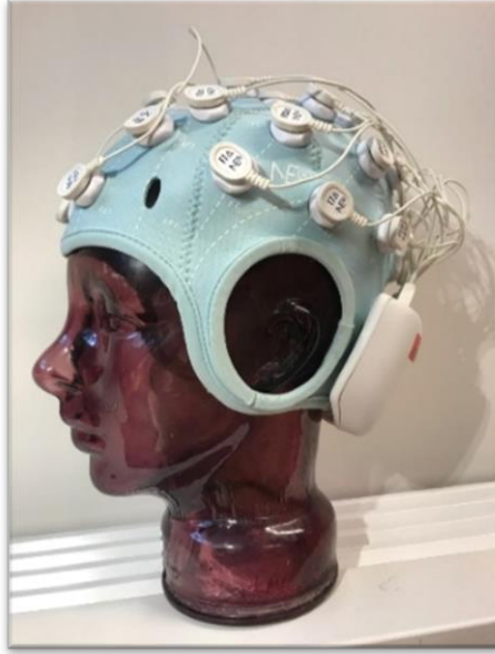
Figure 3. Starstim 32 system (Neuroelectrics, Spain) mounted on a NE056 Headcap R (Neuroelectrics, Spain).
