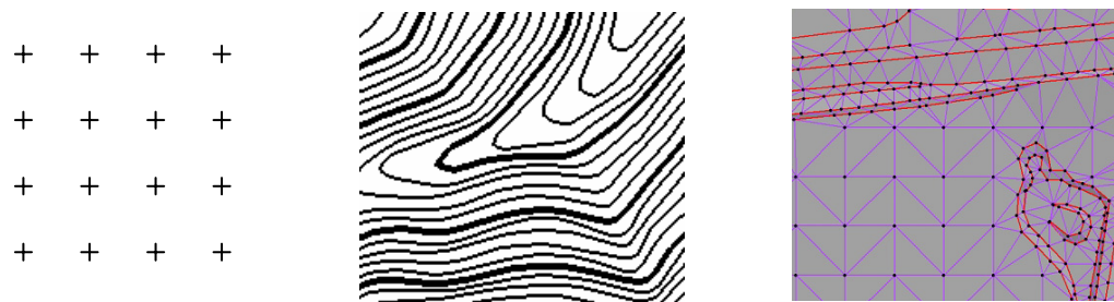
Fig. 3.1 DTM representation by a square mesh regular grid (left), contour lines (middle) and TIN (right). Break lines in TIN are marked with red color.
