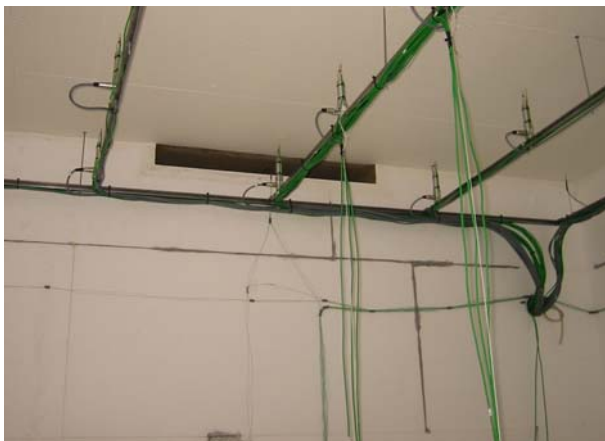
Figure 3. Opening used as air inlet for mixing ventilation and outlet for displacement ventilation.
