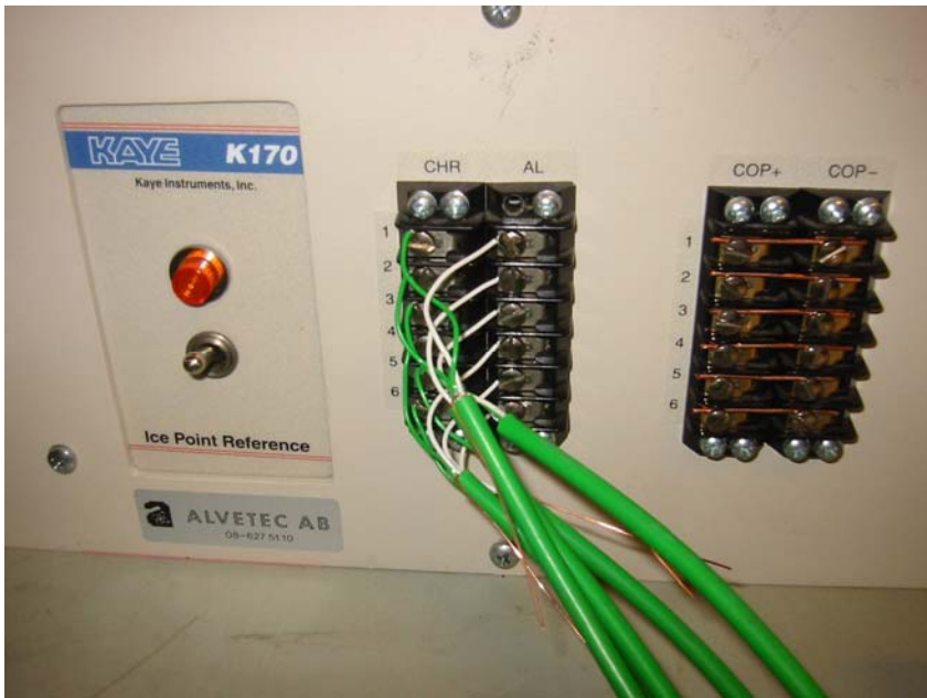
Figure 10. KAYE K170-6 ice point reference with thermocouples connected to the CHR/AL inputs and COP outputs short-circuited.
