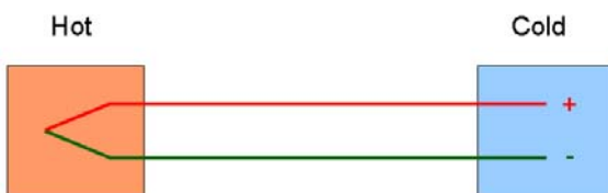
Figure 1. Functional principle of thermocouples
