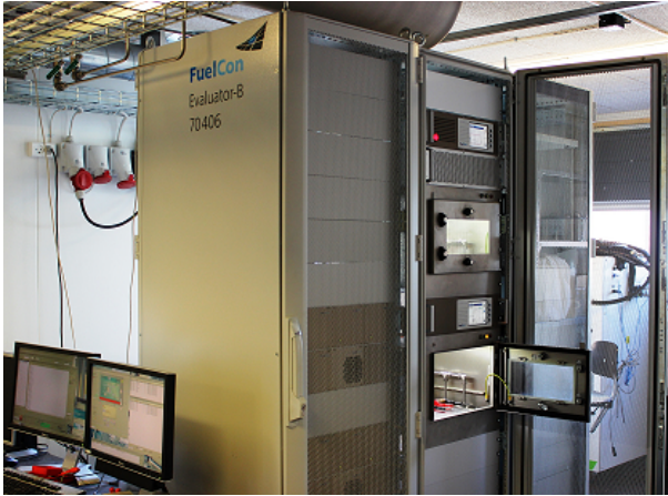
Figure B.1: FuelCon battery test station.
