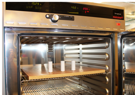
Figure B.4: LFP/C battery cells placed inside one of the Memmert UNPP 500 universal ovens.
