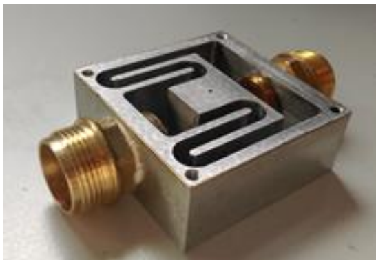
Figure 6-5 TEG cold side heat exchanger with labyrinth view for water path.
