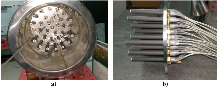
Figure 6-3 a) Front view and b) side view of the heater plate with blowing-air type igniters attached.
