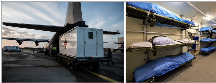
Figure 2.10. Loading of an intensive care module (MEDEVAC module) into a Hercules C-130J Aircraft (left image). The right images shows the interior of the module with patient bays along the walls. (Study 3)
