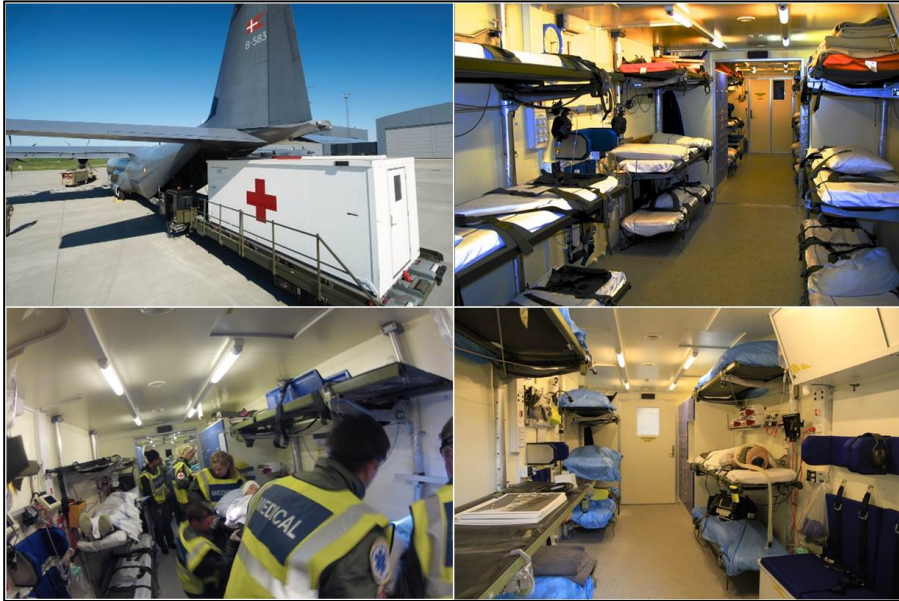
Figure 6.1. Intensive care MEDEVAC module - exterior and interior (photos courtesy of Jean-Michel Ferrieux).
