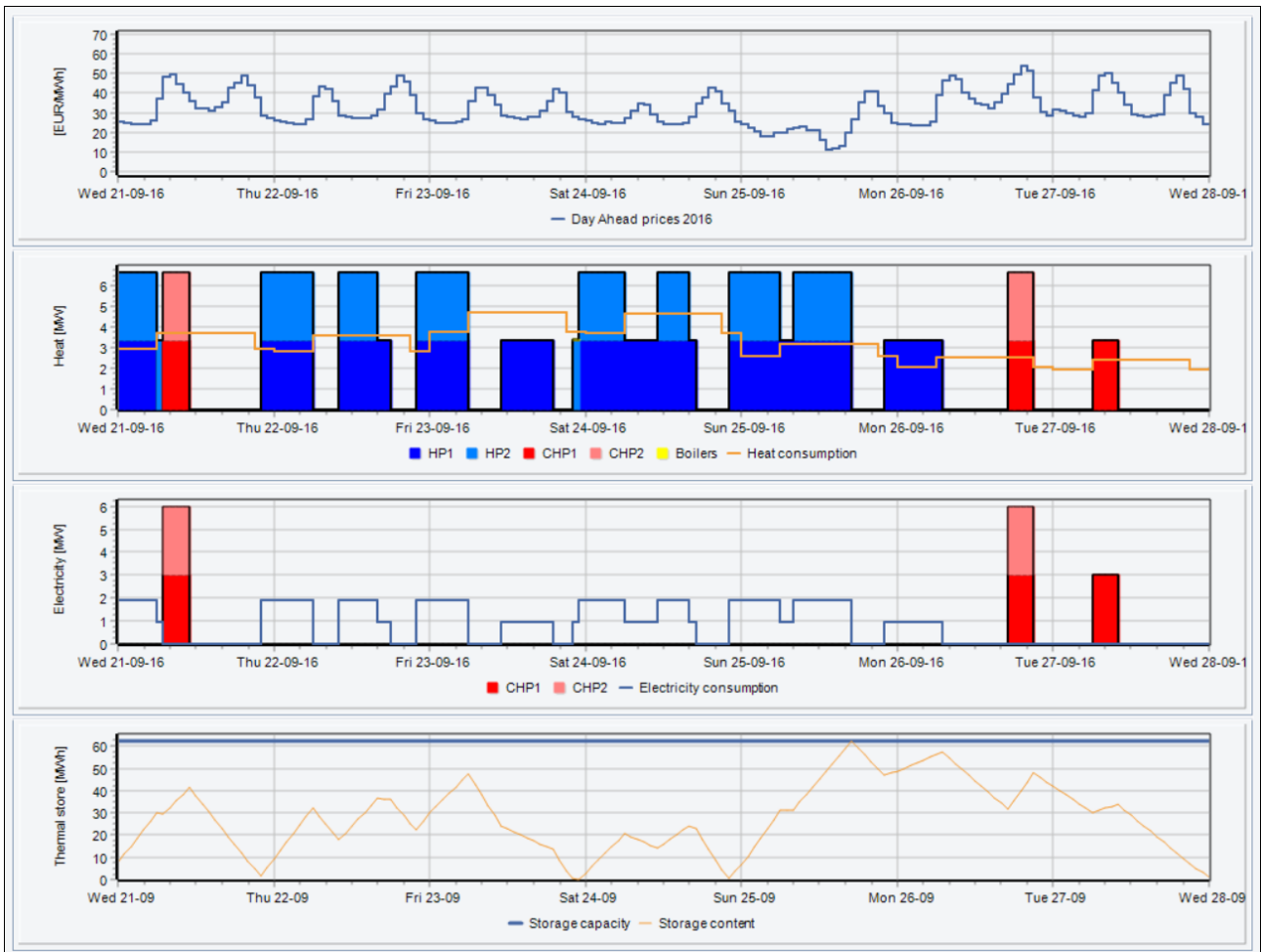
Figure 10: An example of the UC at the DE plant during 7 days in September calculated using the advanced analytic UC method.
