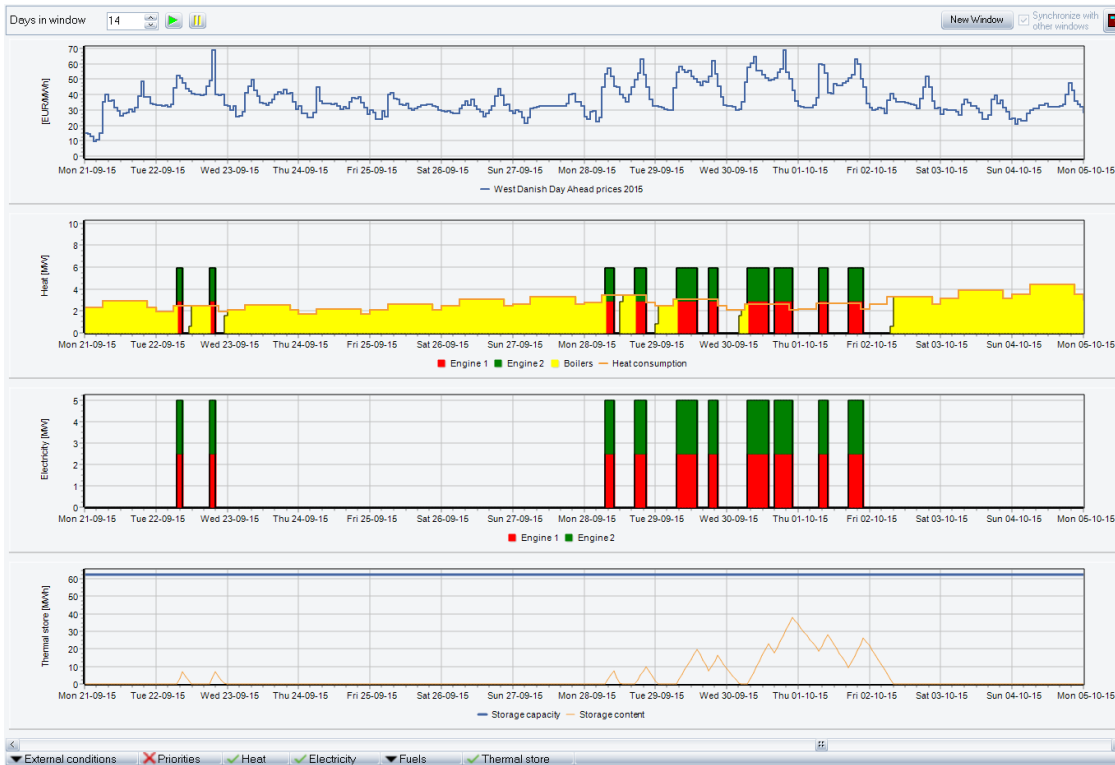
Figure 3: Simulated operation against the Scandinavian day-ahead market in two weeks in the autumn of 2015 of a CHP-plant equipped with large electrical capacity and large thermal store. The simulation is made in the energy systems analysis tool energyPRO [34].
