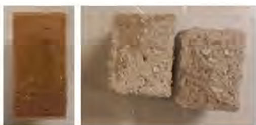
Fig. 14. Penetration depth of agent F on brick and mortar.
