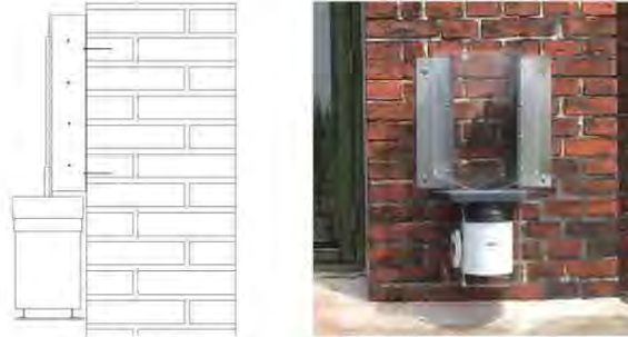
Figure 5: Wall-mounted WDR gauge with HOBO logger. Illustration (left) shows fixation and extension from surface. Image (right) illustrates fixation to façade (test building 1)
