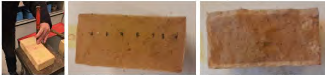
Fig. 3. Halving of brick specimens with hammer and chisel (left), marking of 7 measuring locations on both sides (agent I), and example of visible penetration depth, the lighter area around the brick (agent E).
