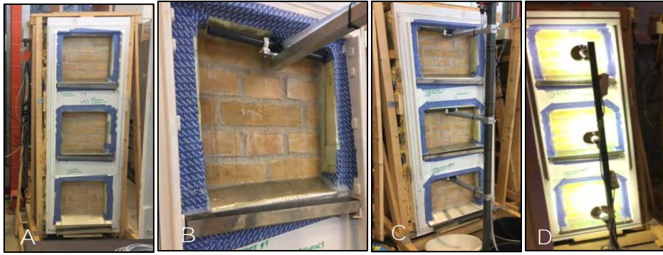
Figure 19: Experimental setup. A: 3 wall sections in mounted in a refrigerator door. B: water loads applied horizontally to the top of the wall section, by perforated pipe. C: view of water loads applied to 3 wall sections. D: radiation loads on 3 wall sections.
