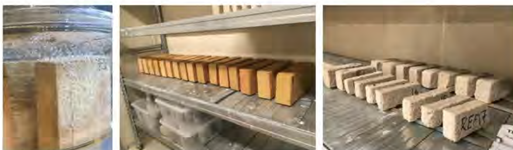
Fig. 2. Vacuum saturation of brick in desiccator (left), and drying in climate chamber of brick (middle) and mortar (right).
