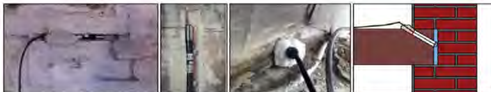
Fig. 1. Sensor locations. From left to right; sensor in existing joint, purposely designed notch and in hole through beam end.
