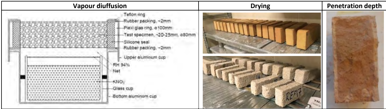
Figure 21: Experimental setups for; vapour diffusion: the principles of the cup setup, drying experiment: brick and mortar specimens in climate chamber, and penetration depth: example of visible penetration depth
