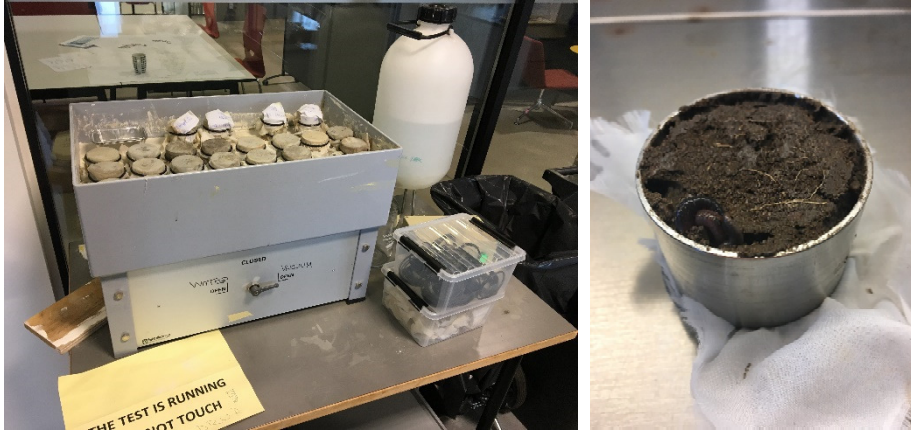
Figure 2.3. Left: Retention box for analysis of intact samples. Right: Intact sample of soil with a live earthworm.
