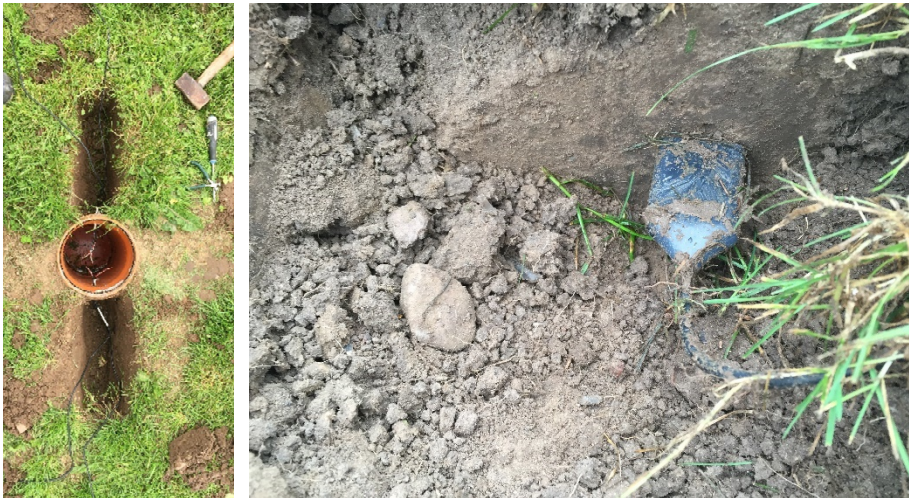
Figure 2.8. Parts of a soil sensor cluster. On the left, a vertically burried \text{\O}200 contains the data logger to collect all data from installed sensor. On the right, a mounted Decagon 5TE soil volumetric water content sensor is seen.
