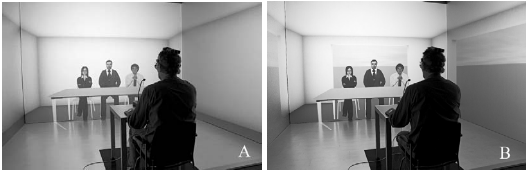
Fig. 1. A participant in front of the committee in the closed room (A) and the open room (B). Due to the stereoscopic projection, the participant will experience a clear 3D environment.
