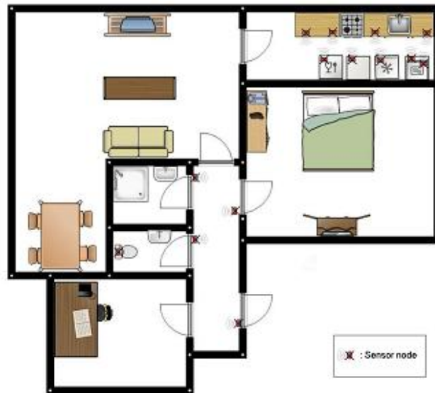
Figure 8.19. The Kasteren et al. (2008a) experimental house equipped with 14 sensors (red crosses).
