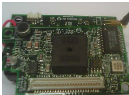
Fig. 1.2: A wireless sensor node
