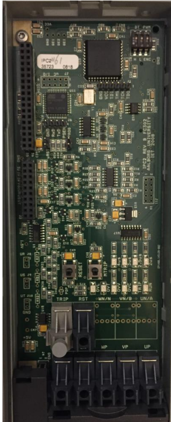
Figure 3.8: Picture of inverter interface board.
