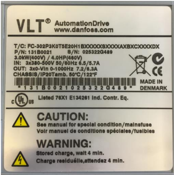
Figure 3.7: Nameplate of inverter.
