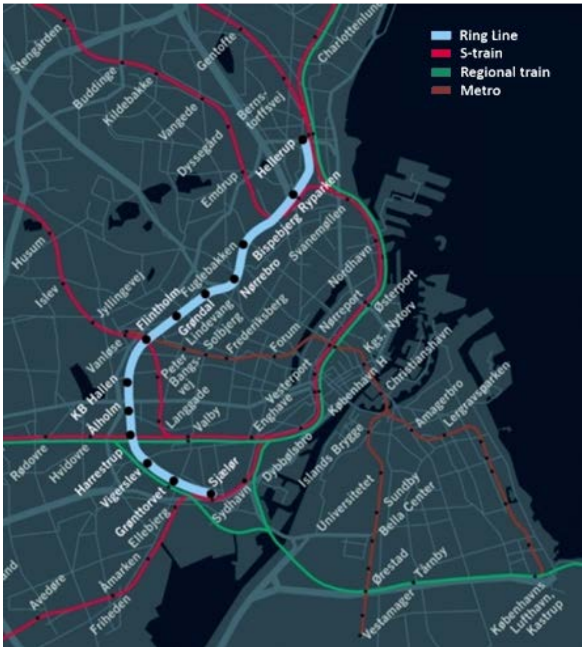
Figure 40: The suggested alignment for Ringbanen prior to passing the construction law. Apart from moving and renaming some of the stations slightly, no changes have been made to the overall design of the project. Reprint from Pilegaard and Johnsen (1999), translated by the author.
