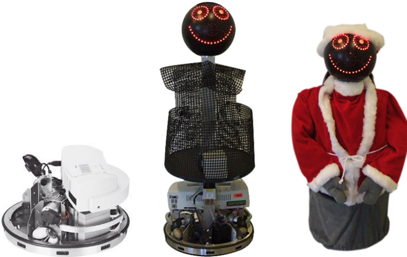
Figure 6.1: Left: The original robot platform from FESTO. Center and Right: The modified platform by AAU called Robotino
