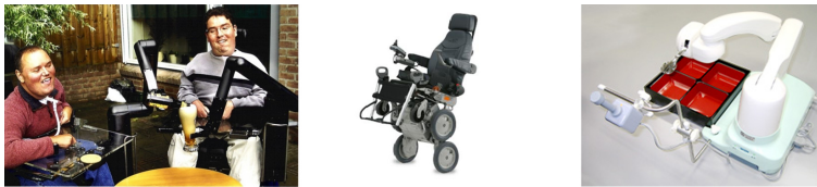
Figure L.2: The iARM from Exact Dynamics [3], the iBOT wheelchair [4] and the mySpoon robot [5]
