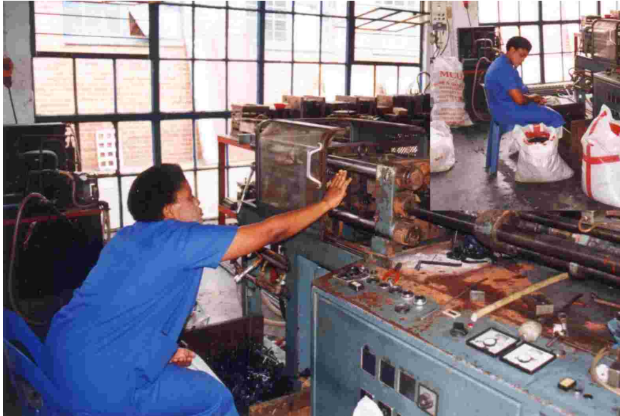
Figure 45 Operator intervenes frequently in order to release jammed item in injection moulding machine
