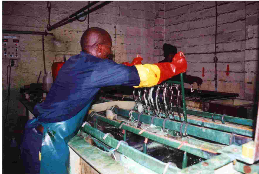
Figure 40 No hoist is installed in the subsequent rinse steps
