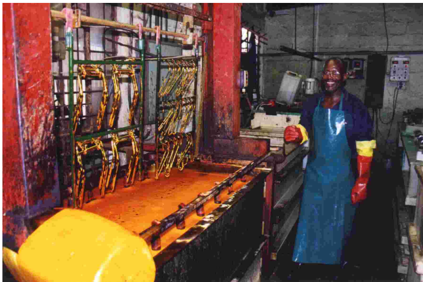
Figure 39 A slow hoist enhances drip off and reduces lifting strain
