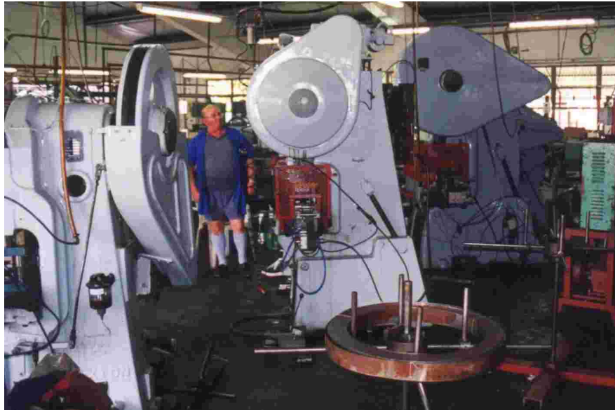
Figure 44 Noisy power presses located in the middle of a large production hall
