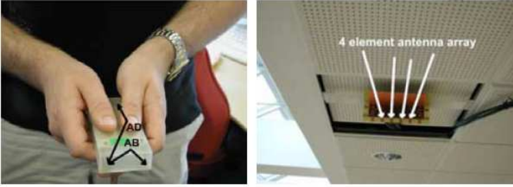
Figure 1: Antenna setup for the measurement setup, left: handheld user device (UD); right: access point device (AP)
