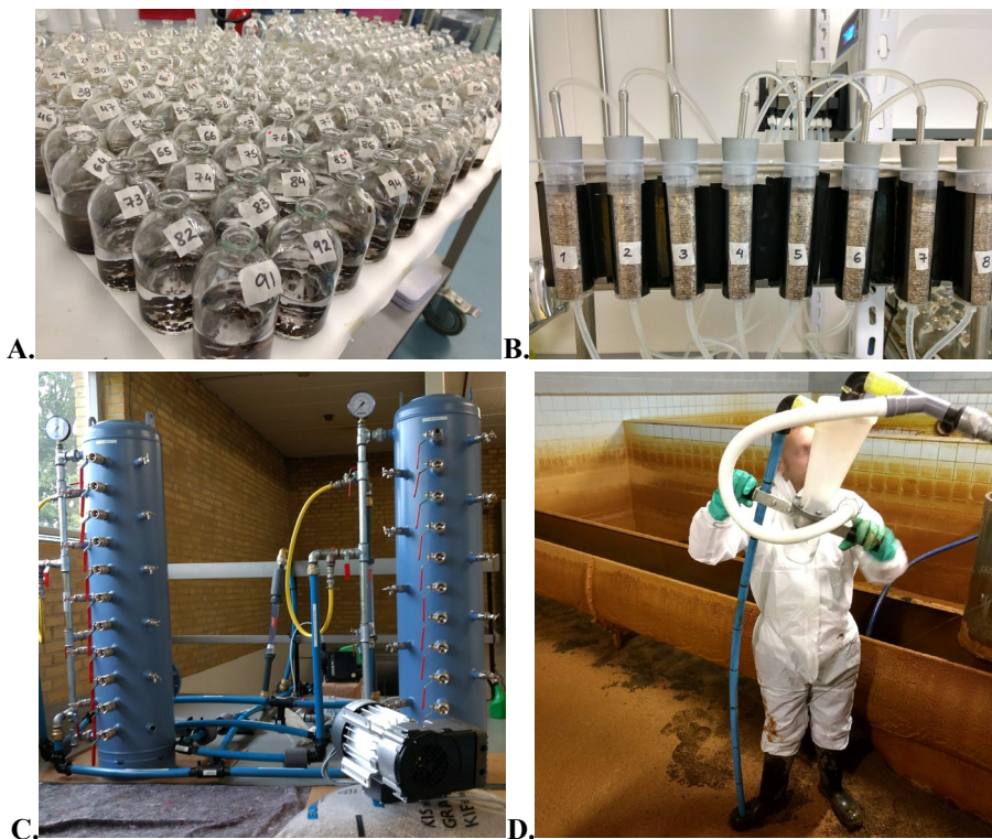
Figure 14 Photographs of A. batch-scale assay B. column-scale assay C. pilot-scale assay designed in collaboration with Silhorko-Eurowater A/S D. sampling from a full-scale filter at a DWTP.
