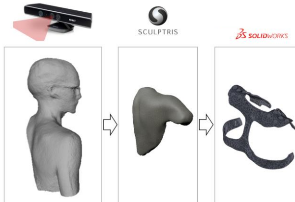
Figure 1-2. Workflow for design custom-fitted orthosis parts. From a 3-D point cloud of a scanned shoulder region to a comfortable fitting cuff.
