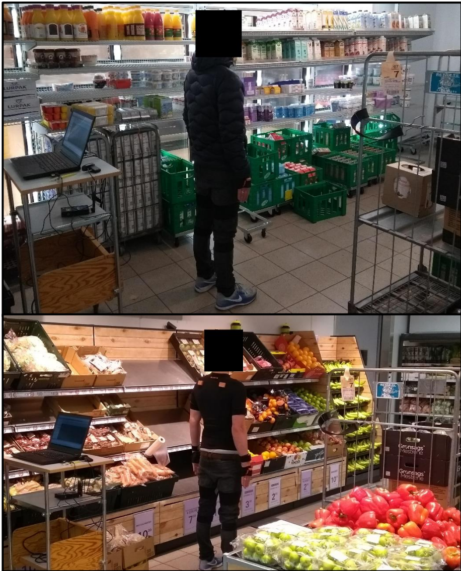
Figure 2.1 – Illustration of the experimental procedures for Experiment II. The subject is standing in a neutral posture during the calibration of the inertial motion capture system prior to performing MMH tasks in the meat and dairy (top) and fruit and vegetables areas (bottom). The surface electromyography electrodes are hidden under the subject's clothes.
