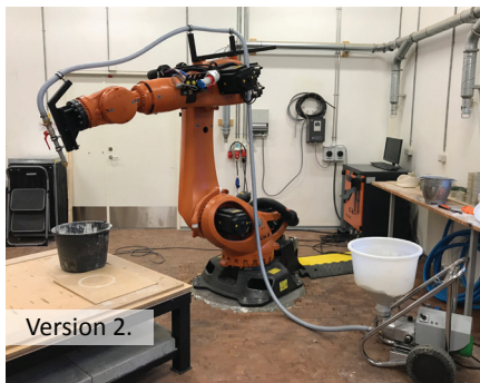
Figure 4.3. Development of prototypes for the concrete extrusion system. Version 1: Linear actuator ram originally designed for clay extrusion, by www.3dpotter.com Version 2: Peristaltic pump from Köster connected to a custom nozzle with a single hose. Version 3: A concrete pump from MAI with a custom nozzle for direct extrusion without hose. Final version: Setup with two concrete pumps from MAI. A 'feed pump' at the floor connected with hoses to an 'extrusion pump' mounted on the robot arm. Photos by Mads Brath Jensen
