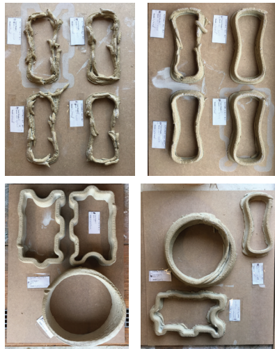
Figure 4.4. Experiments with the concrete material system. Several extruded prototypes were fabricated to investigate the connection between nozzle size, extrusion flowrate and material mixing ratios. Photos by Mads Brath Jensen
