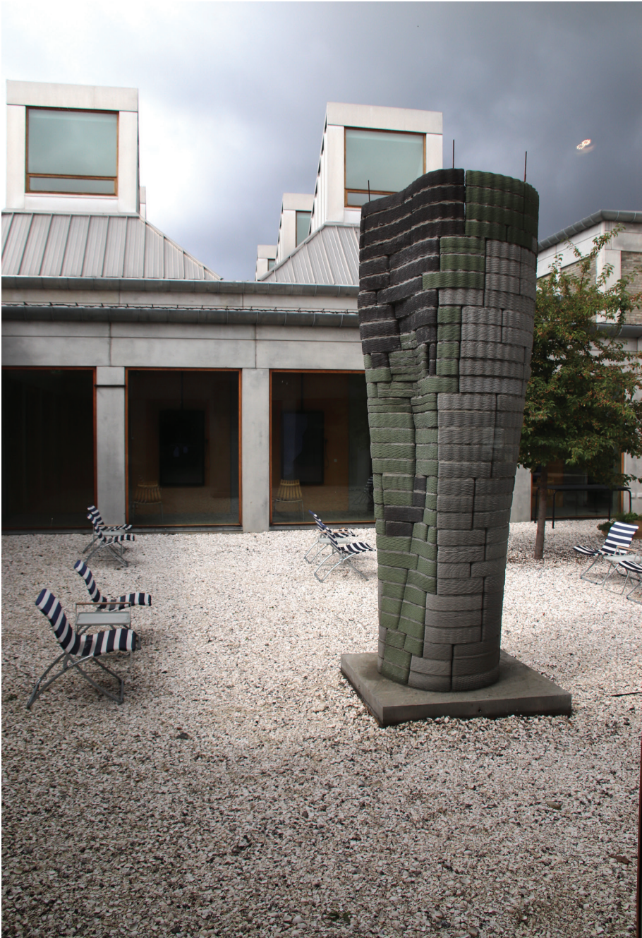
Figure 4.1. The full scale concrete demonstrator assembled in the court yard of the Utzon Center, Aalborg, Denmark. Photo by Mads Brath Jensen.
