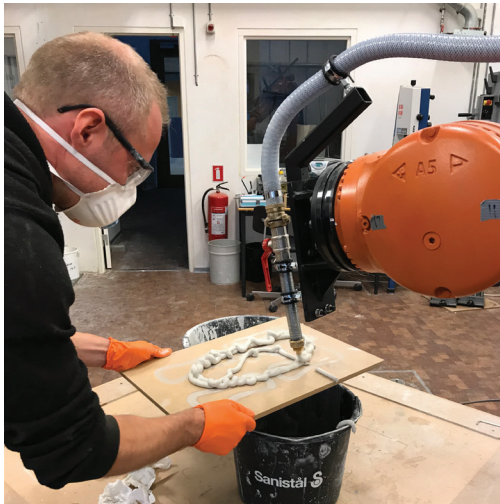
Figure 4.4. Experiments with the concrete material system. Several extruded prototypes were fabricated to investigate the connection between nozzle size, extrusion flowrate and material mixing ratios. Photos by Mads Brath Jensen
