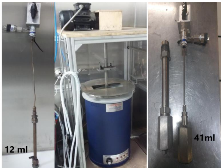
Figure 3. The reactor system in HTL experiments
