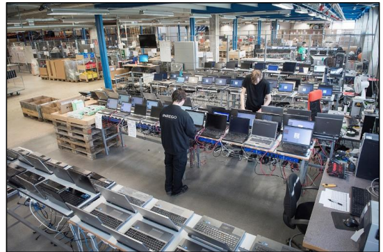
Figure 12: View of the testing and data erasing line at Inrego. Image provided by Inrego
