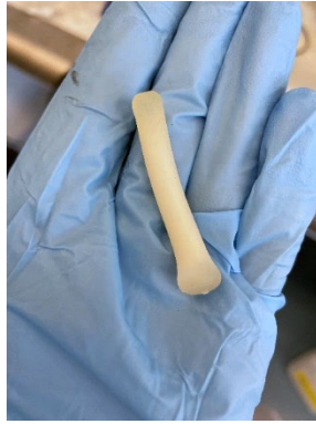
Figure S8. M-DIPN hydrogel is unable to adhere to any surface.
