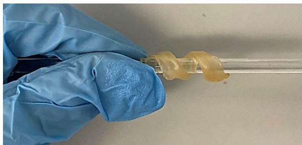
Figure S4. Wrapped d-DIPN hydrogel around a glass rod.
