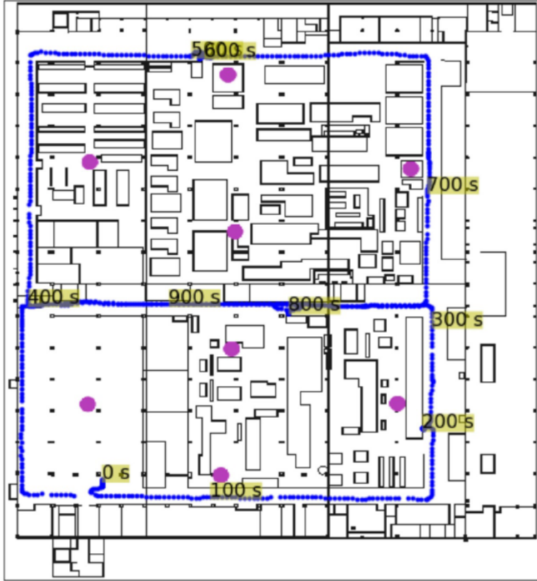
Fig. F.7: Factory shopfloor plan, deployment of the 5G RRHs, and an AGV route across the factory hall.
