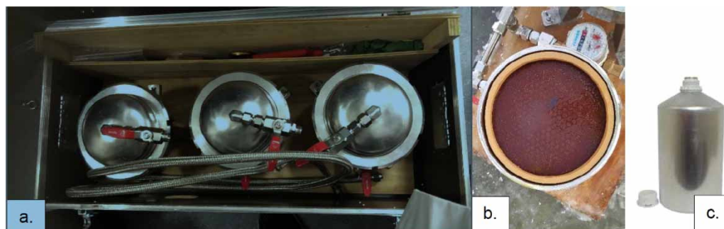
Figure 1 | The filtering unit with metal tubing and metal pump head (a), metal filter (b), and aluminum sampling container (c).
